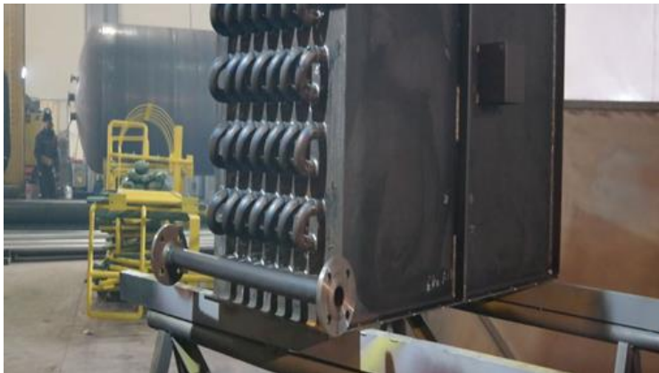
Boiler Feedwater economizer
